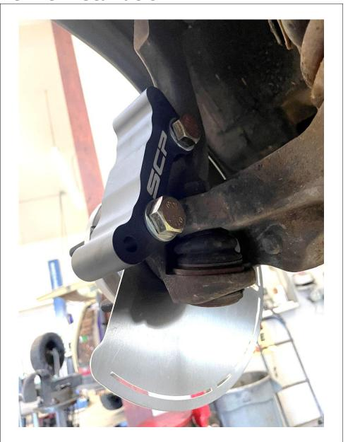
8. The disc, caliper assembly, and 3/8" bolts/washers must be installed as one assembly. Insert the 3/8" bolts with washers under their heads into the calipers pointing towards the inside of the van. Slide the caliper assembly over the disc. Then, install the assembly as shown to the right. You are aligning all 5 wheel studs and both 3/8" bolts so this can be a bit finicky.
