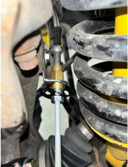
13. Now bend the hardline and thread it into the fitting installed in the caliper. A Syncro example is shown in the left image and a 2WD example is shown in the right image.
