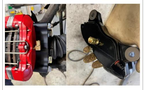
5. Remove the allen socket bolt that retains that brake pad sliders.
