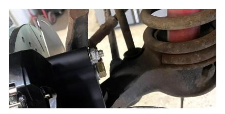
10. Install the female to female brake line union to the male end of your stainless steel brake hose.
