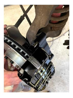
9. Install a 3/8" washer and a vibration resistant lock nut on each of the 3/8" bolts. Torque to 35 ft-lbs.
