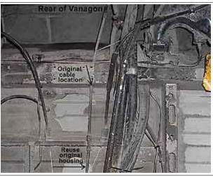
4. On the front passenger side of the engine compartment (some models only), there is an existing inverted "V" shaped slot in the sheet metal. The cable bracket can be positioned in the slot and a sheet metal screw used to attach it. If no slot is present, simply drill appropriate holes in the lower part of the firewall. Try to leave a nice gentle curve from there to the engine connection.
