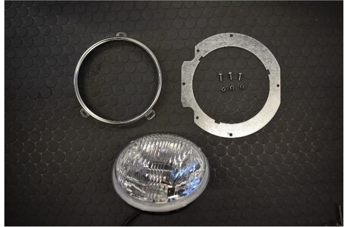
2. Line up the backing to the tabs on the back of the headlight. The cutouts on the retaining ring should be at the top of the headlight.
