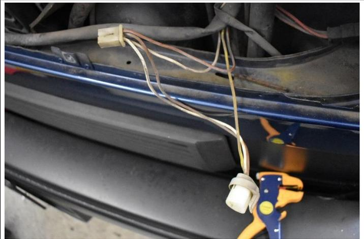
3. Take the supplied H4 harness and cut the male connector off the end. Be sure to mark which wire went to which pin of the H4 connector. Now connect the supplied harness to the three stripped wires on the van using the supplied crimp connectors. The diagram to the right shows which wires go to which. Colors of wire on your H4 harness may vary so reference the pins and not the wire color.
