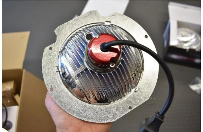
3. Place chrome retaining ring over headlight and align the holes. They will only align one way. Install the 3 screws and nuts through the three aligned holes. Tighten completely.
