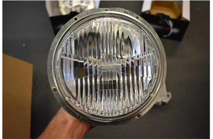
5. Find your 3 M5 bolts and 3 springs. Slide your bolts through the remaining holes on the top and sides of the assembly. Slide the three springs over each bolt.
