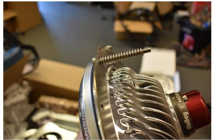
6. Place the assembly onto the housing bracket and start each of the three screws. Remember, you need to create a left and a right assembly so one assembly needs to be the mirror image of the other. Only tighten the screws down to the point that the springs are slightly in compression.
