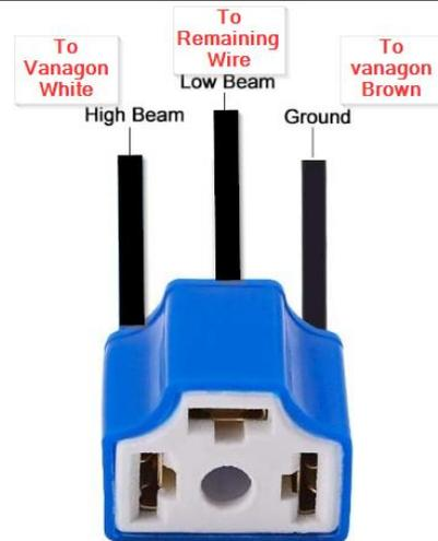
4. If you only want your inner headlights to act as high beams, cut and terminate the wire going to the low beam pin of the H4 connector for the inner headlights. See the diagram above for this pin location.
