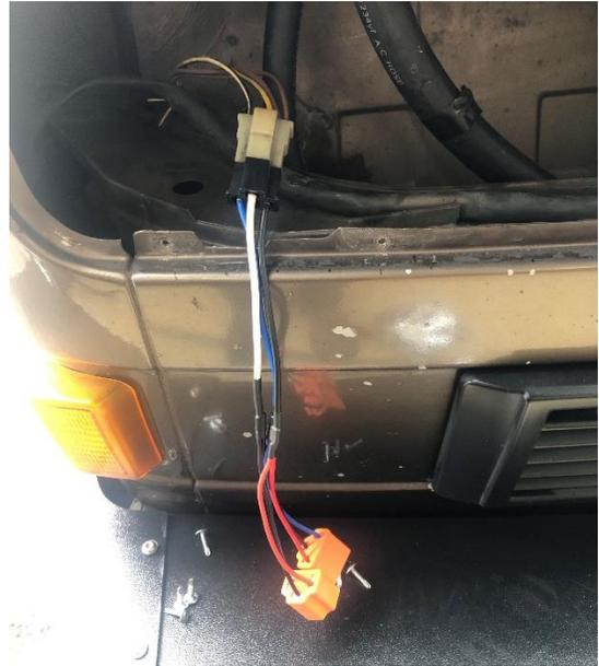
3. If you only want your inner headlights to act as high beams, cut and terminate the wire going to the low beam pin of the H4 connector for the inner headlights. See the diagram to the right for this pin location.
