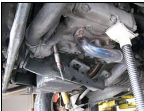
Figure 7: Unbolted Subaru oil pan and right side engine mount. Engine is supported by jack.
