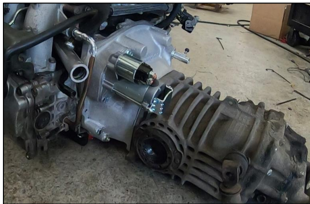
Figure 16: Completed installation of a manual Vanagon transmission to an EJ25 using Small components.
