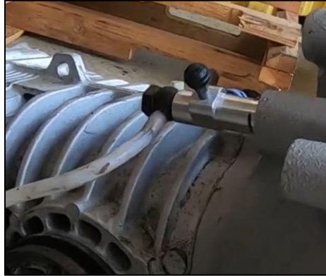
Figure 17: Post-1985 Vanagon with banjo fitting installed onto release bearing hydraulic fitting.
