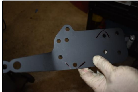
Figure 11-7: Throttle pedal bracket with holes that will be used marked.
