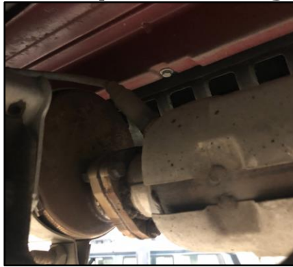
Figure 52: Installed second catalytic converter with Subaru oxygen sensor installed.
