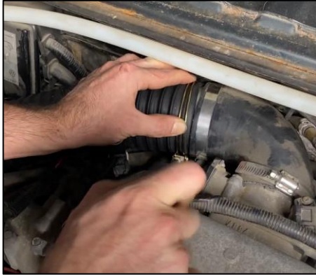
Figure 60: 3 Inch intake tubing install to intake manifold elbow.
