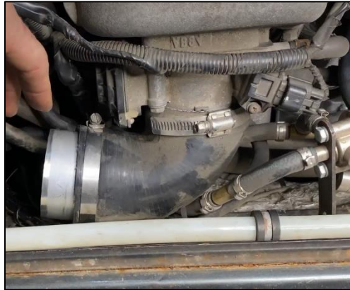
Figure 56: Installed reduce elbow and aluminum coupling. Elbow must point towards driver's side.
