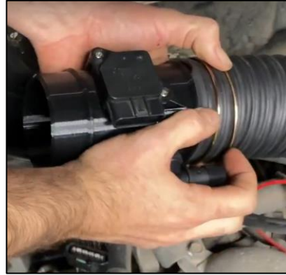
Figure 61: 3 Inch intake tubing install to MAF Sensor coupling.
