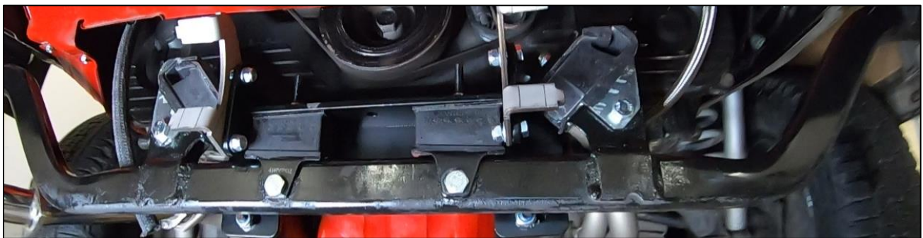
Figure 3: Installed EJ25 motor with Small Car Motor Mounts and stock Vanagon rubber mounts.
