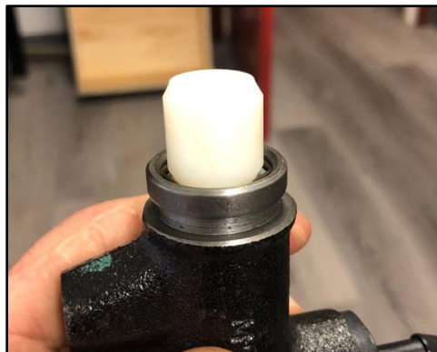
Figure 18: Master cylinder with boot removed and spacer placed in position for illustration purposes only.
