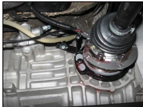
Figure 21: Installed speed sensor on a manual Vanagon transmission.
