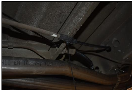
Figure 27: Fuel line installed to act as a coupling between new and old throttle cable tubing.
