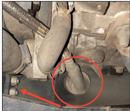
Figure 2: Passenger side engine mount and Small Car oil pan must be installed/removed at the same time.
