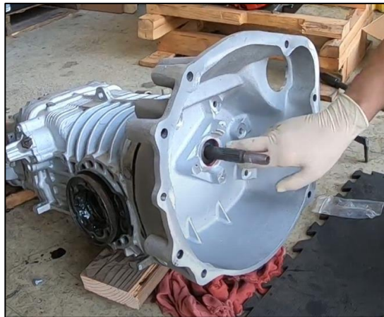
Figure 12: A mated bellhousing with a properly installed input shaft seal
