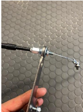
Figure 11-11: Throttle cable installed to bracket.
