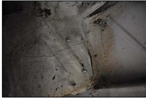
Figure 35: Wheel well view of bolts used to mount accelerator pedal.
