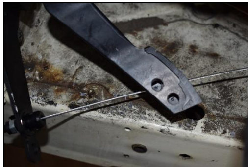
Figure 11-12: Cut and drill Subaru accelerator pedal.
