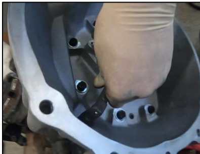
Figure 14: Release bearing install into bellhousing.
