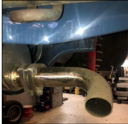
Figure 54: Installed tail pipe.
