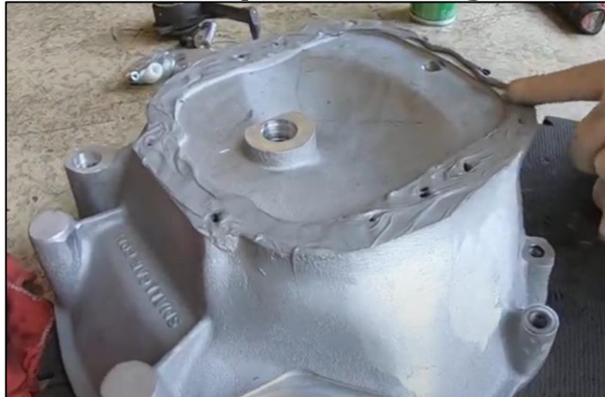
Figure 13: Permatex Ultra Grey applied to the mating surface of the Small Car Bellhousing.
