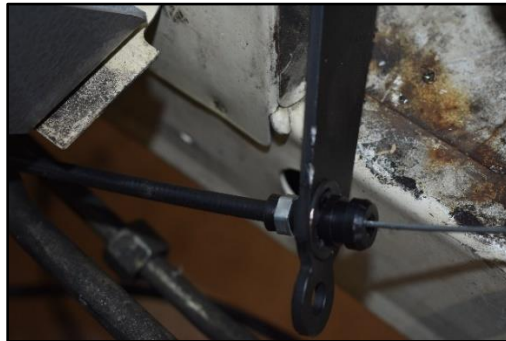
Figure 36: Throttle cable installed to bracket.
