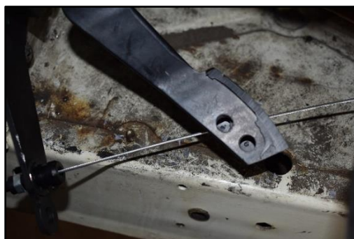
Figure 37: Cut and drill Subaru accelerator pedal.
