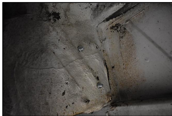
Figure 11-10: Wheel well view of bolts used to mount accelerator pedal.
