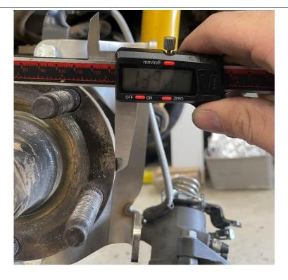
3. Install your hub. The hub castle nut must be torqued to 253 ft-lbs then secured with a cotter pin. See Bentley for more details on this install.
