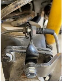
11. Now take your new parking brake cable and hook it to the caliper as shown to the right. Then, loose the parking brake cable tensioner in the center of the van, hook the new parking brake cable into it, and tighten the tensioner until the parking brake is well adjusted.
