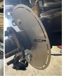
5. Install the two M10X20 bolts into the threaded holes on the bottom of the bearing housing. Then, install the M10X30 bolt, washer, and lock nut.
