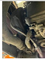
**3.** Secure the dipstick bracket to the van so that it is accessible from the license plate hatch. The bracket can be secured with a bolt and rivet nut or a self-tapping screw. The example to the right shows a self-tapping screw install.
