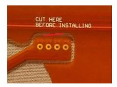
There is a small "bridge" that needs to be cut (with scissors) located at the 4-pin tachometer connector.
