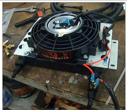
4. Zip-tie the wire and fuse holder to the mounting bracket.
