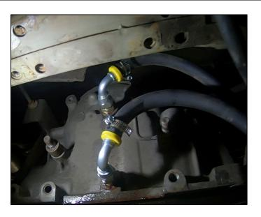
6. Reinstall transmission mount and remove the transmission support. The hoses will route to the right side of the mount when facing the back of the van.
