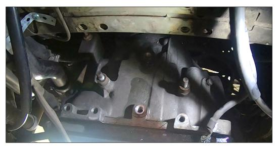
3. Install 12mm A/T fittings with 12 x 16mm copper crush washers.
